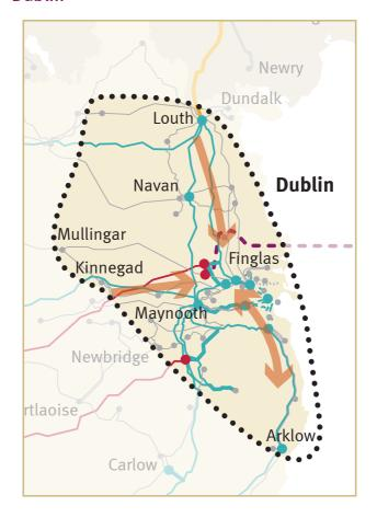
The grid in this region is mainly made up of 220 kilovolts (kV) underground cable and overhead lines, with two 400 kV lines connecting to the rest of the country. Although well resourced, the expected growth in onshore and offshore wind generation will be a challenge.
