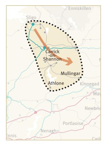
The existing grid in this area uses 110 kV and 220 kV lines, with power flowing west to east through this network. We expect that this area will be challenged during high wind conditions, as anticipated wind farms in the west add more power to the grid.
