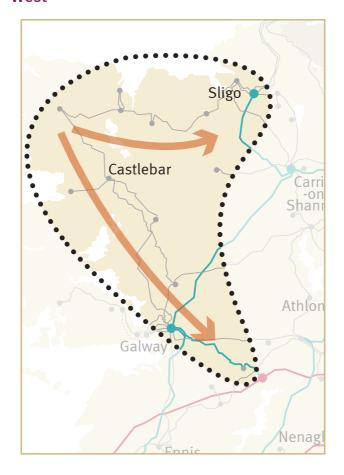
Currently this area of the grid relies on low capacity 110 kV, and has some 220 kV connections to the wider grid. All four scenarios will see this infrastructure at potential risk due to growth in renewable energy sources in the area. The consequences of these new connections will be a lack of capacity to carry this clean energy, and a potential lack of capability to reliably supply the electricity needed. There is a strong need for grid development in this area.
