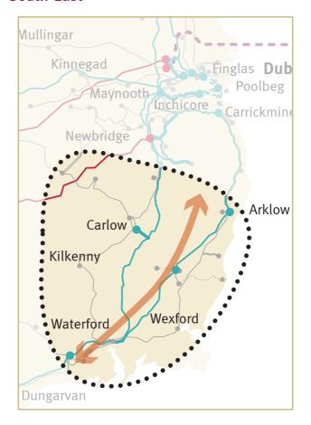
As with other mostly rural areas of the grid today, this area uses 110 kV and 220 kV lines. There is a lot of power moving through this area, with zones of high demand to the north and south of this region. Growth in renewable energy - such as solar and offshore wind - will combine with new interconnection to create a challenge for this area.
