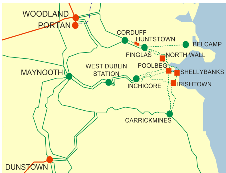
Figure 8-2: Dublin area 220kV transmission system
