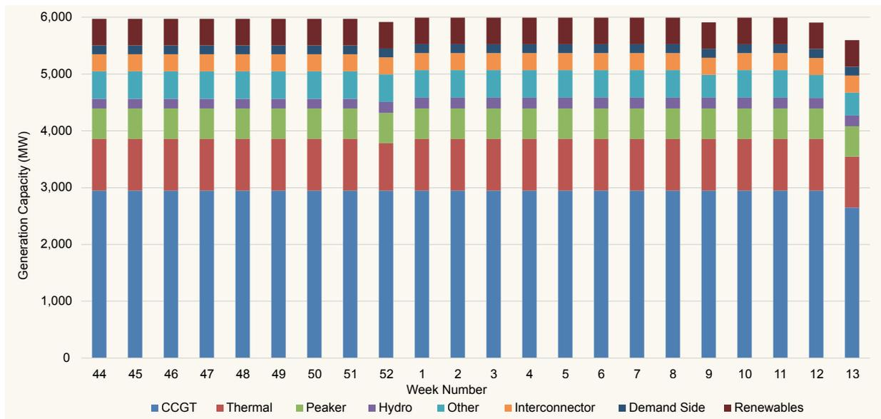
**Figure 13: Ireland expected weekly de-rated generation capacity per type of generating unit**
