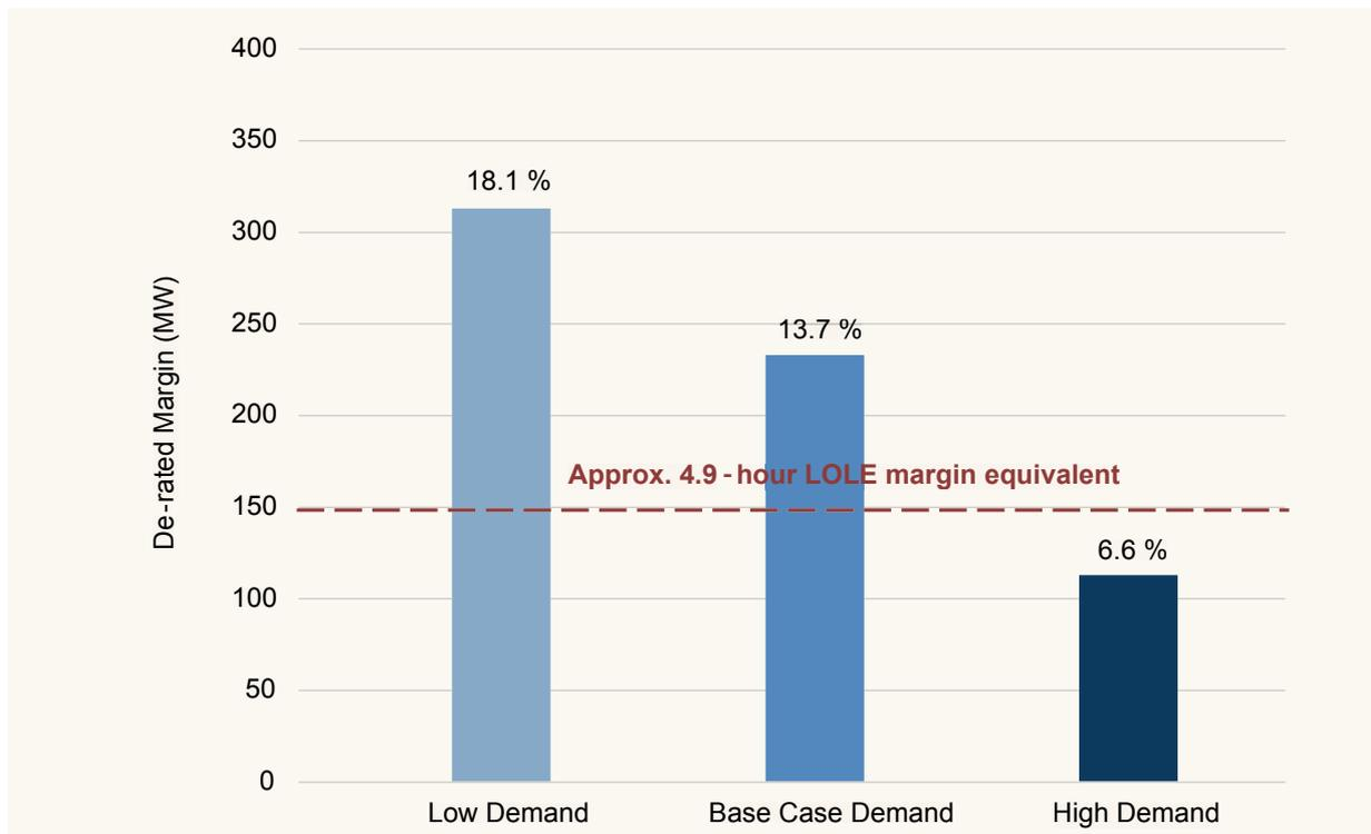
Figure 4: Northern Ireland de-rated margin for low, median and high demand scenarios for the day of lowest capacity margin
