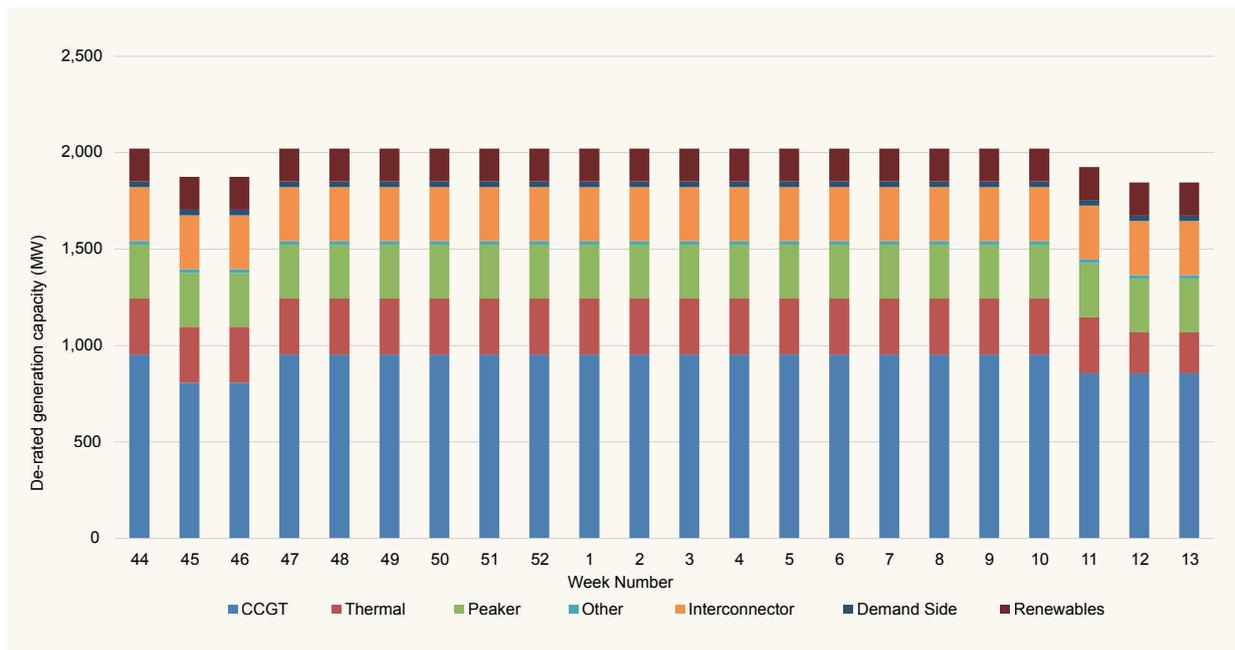
Figure 5: Northern Ireland weekly de-rated generation capacity per type of generating unit
