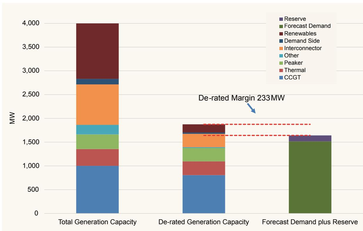
**Figure 3: Northern Ireland generation capacity versus forecast demand for the day of lowest capacity margin**
