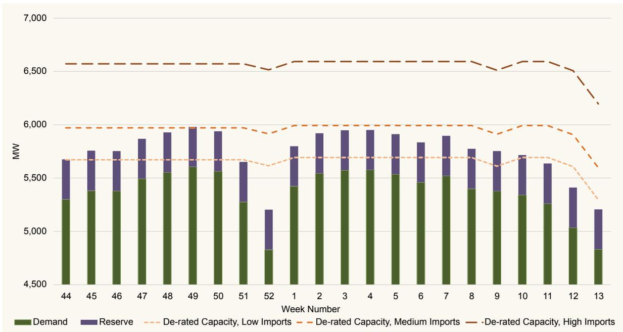
Figure 14: Ireland weekly de-rated generation capacity (dashed lines) for each import scenario versus the forecast demand plus reserve (bars)
