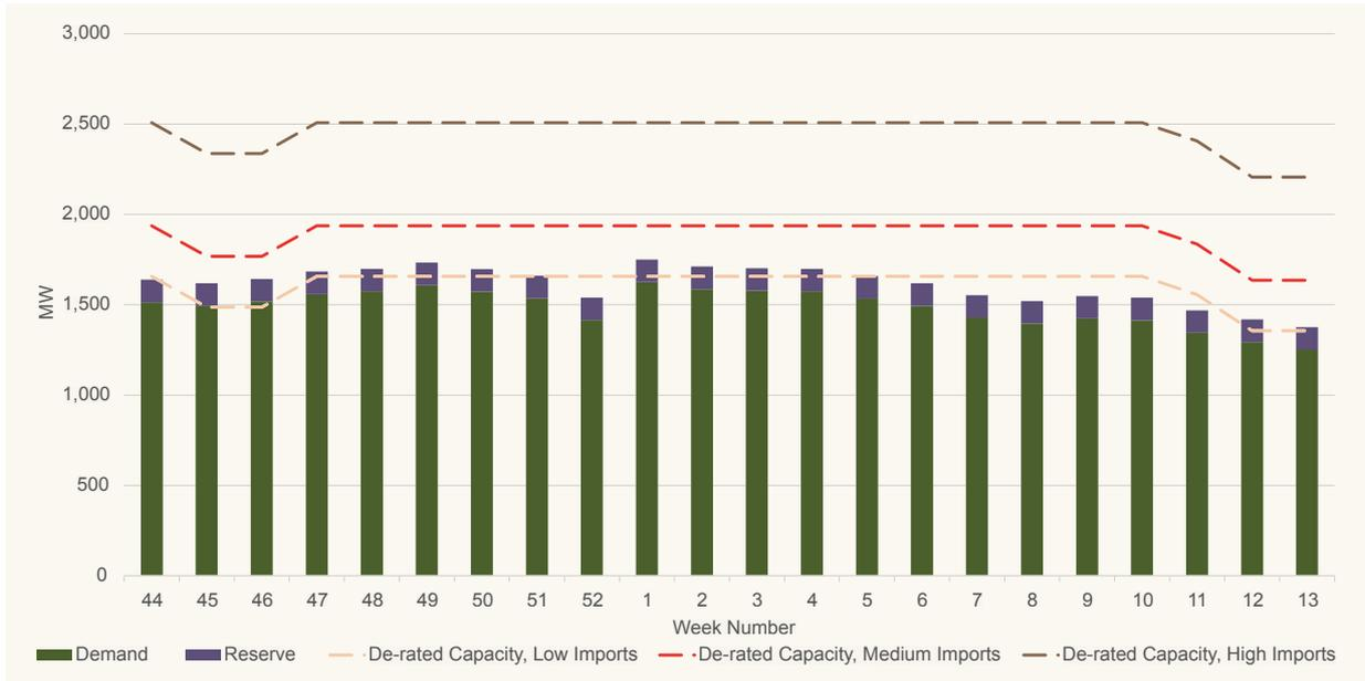
**Figure 7: Northern Ireland weekly de-rated generation capacity based on the largest unit being unavailable (dashed lines) for each import scenario versus the forecast demand plus reserve (bars)**
