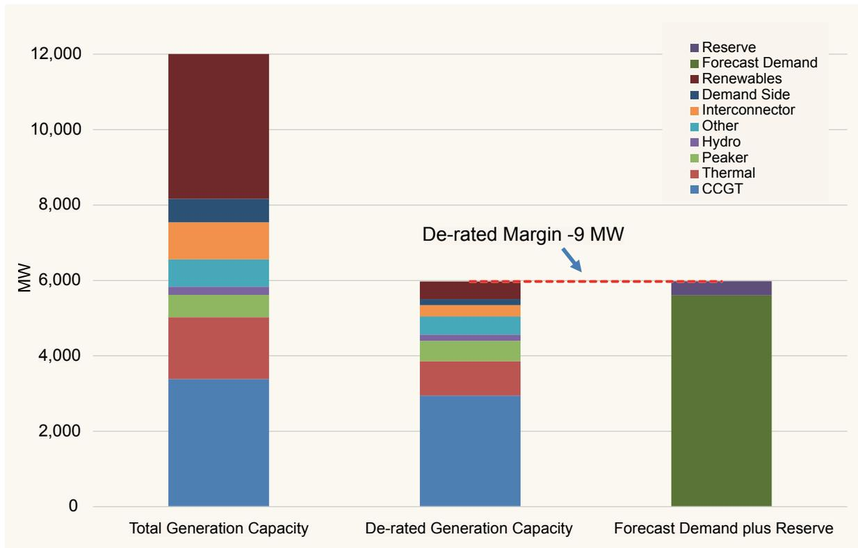
Figure 11: Ireland generation capacity versus forecast demand for the day of highest peak demand / lowest capacity margin
