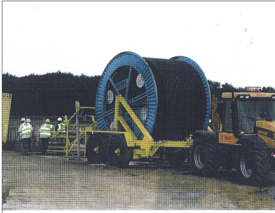
Figure 7 Cable Drum Carrying Trailer
