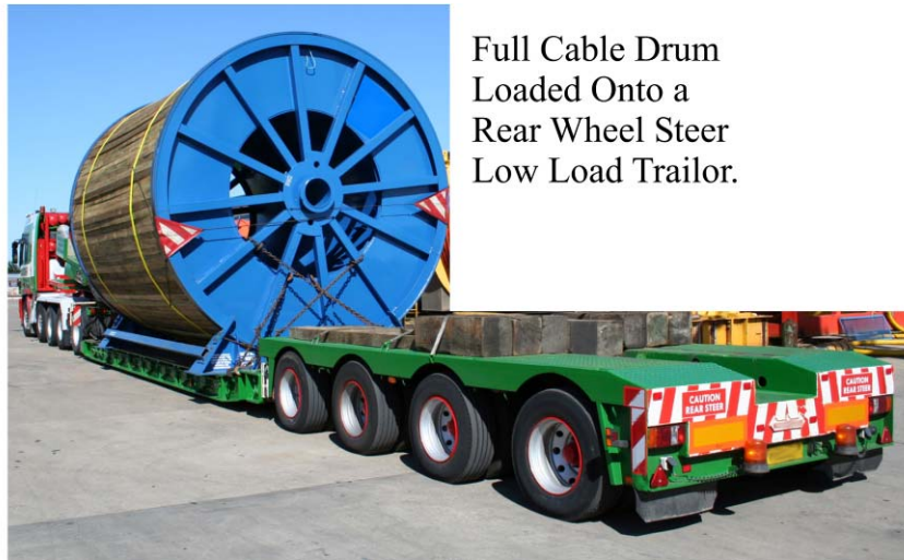
Figure 8 Cable Drum Load Transversely onto a Trailer
