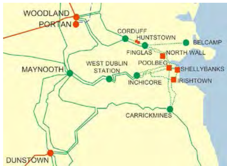
Figure 8-2: Dublin area 220kV transmission system
