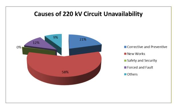
Figure 10: Causes of Unavailability on the 220 kV System in 2021
