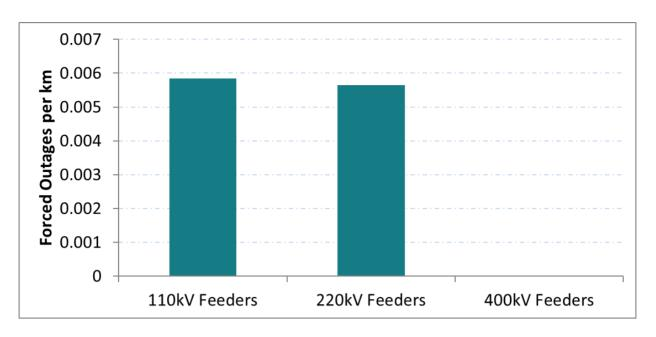
Figure 15: Forced Outages of lines and cables per km in 2021
