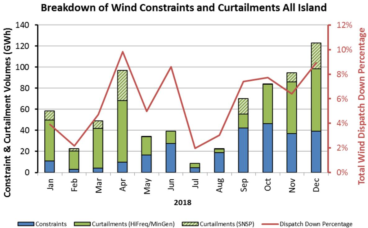
**Figure 2:** Monthly breakdown of the main wind dispatch-down categories on the island in 2018
