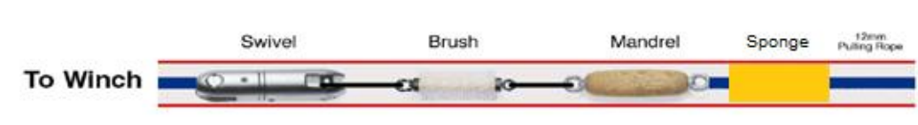
Figure 3 - Set up for Swivel, Brush, Mandrel and Sponge for Duct Proving and Cleaning
