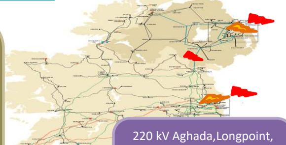
220 kV Aghada, Longpoint, Finglas, and 275 kV Ballylumford - 3PH faults create insecurities when VDIFD is considered.
