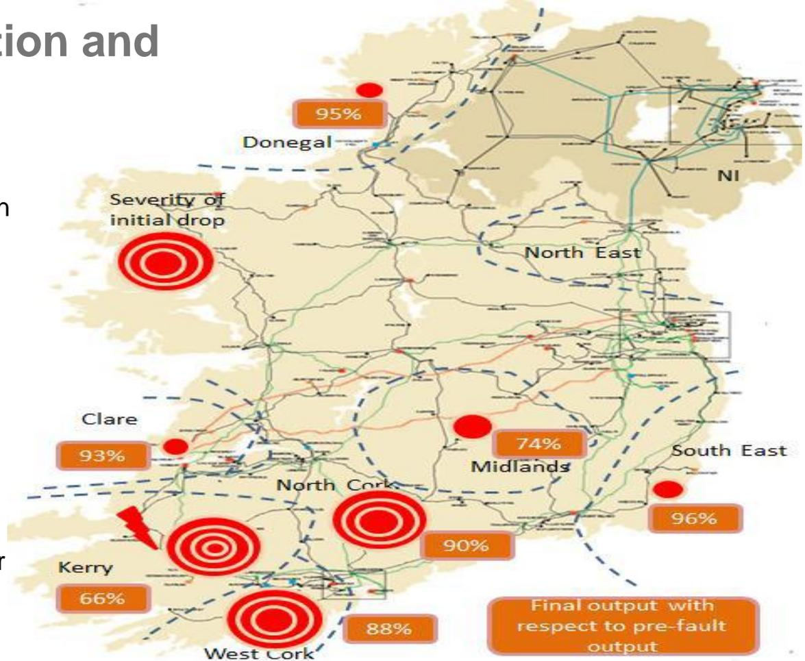
Note: This is an example of VDIFD impact due to WF model with conservative VDIFD response.
