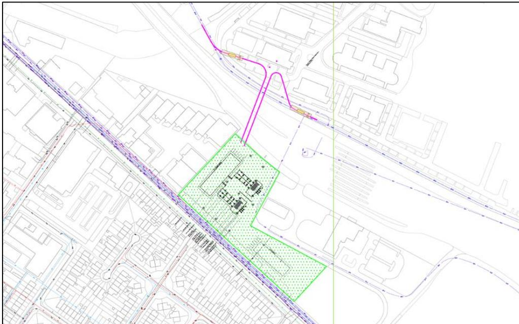
Figure 3-3: Potential Location 1 with adjusted generic substation layout and potential 220 kV tie in
