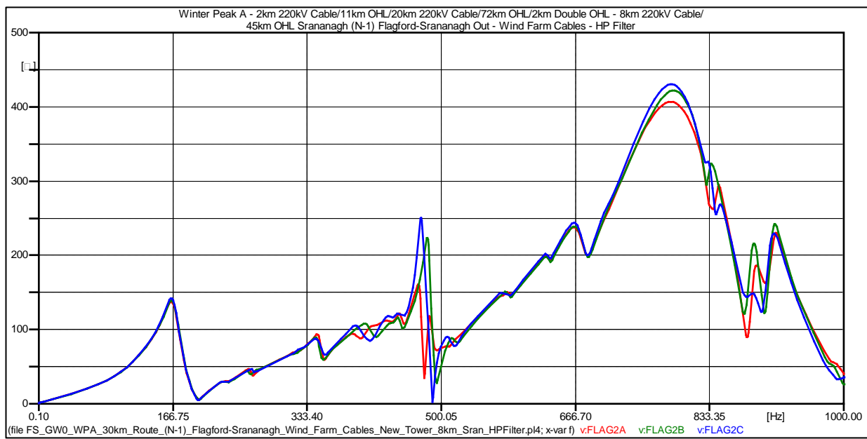
Figure 33: WPA - Length 30 km - (N-1) Flagford-Srananagh Cable/Line Out
