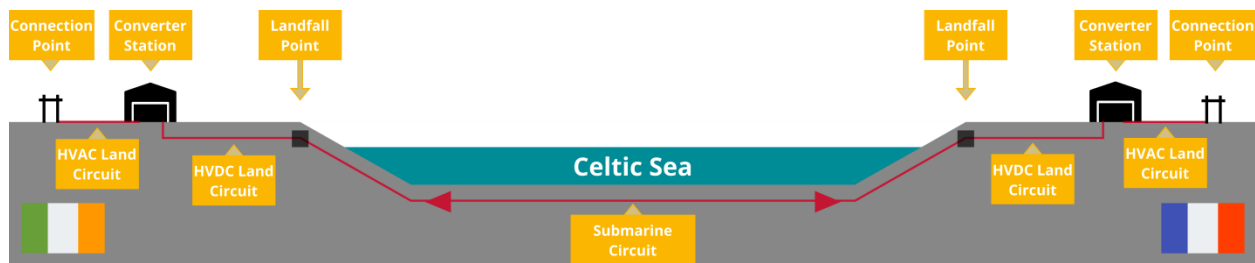
Figure 2 - Illustrative Schematic of the Celtic Interconnector Project
