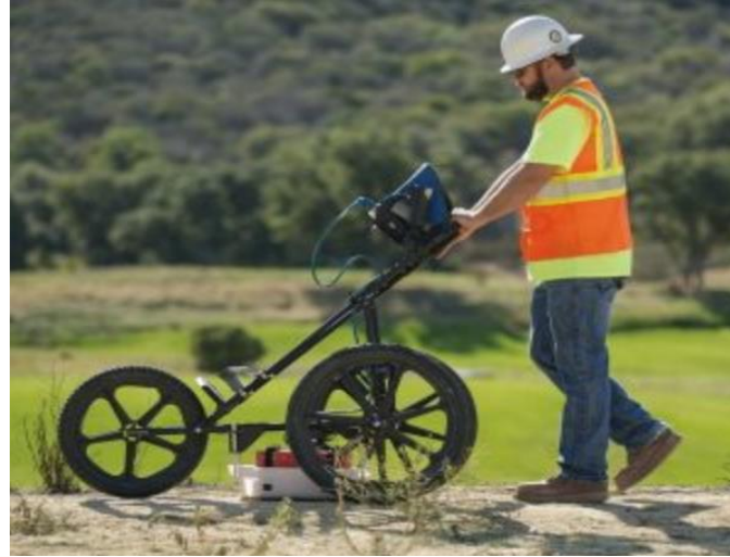
Ground Penetrating Radar
