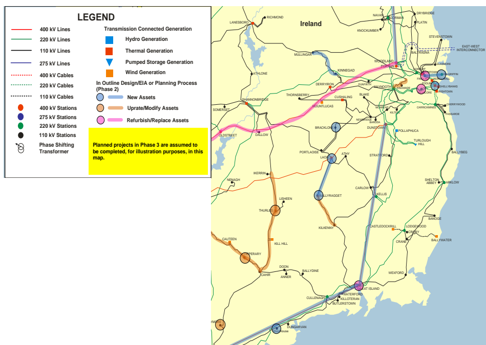
Figure 6-7a Planned Network Developments in the South-East, Mid-East, Dublin Planning Area in Phase 2
