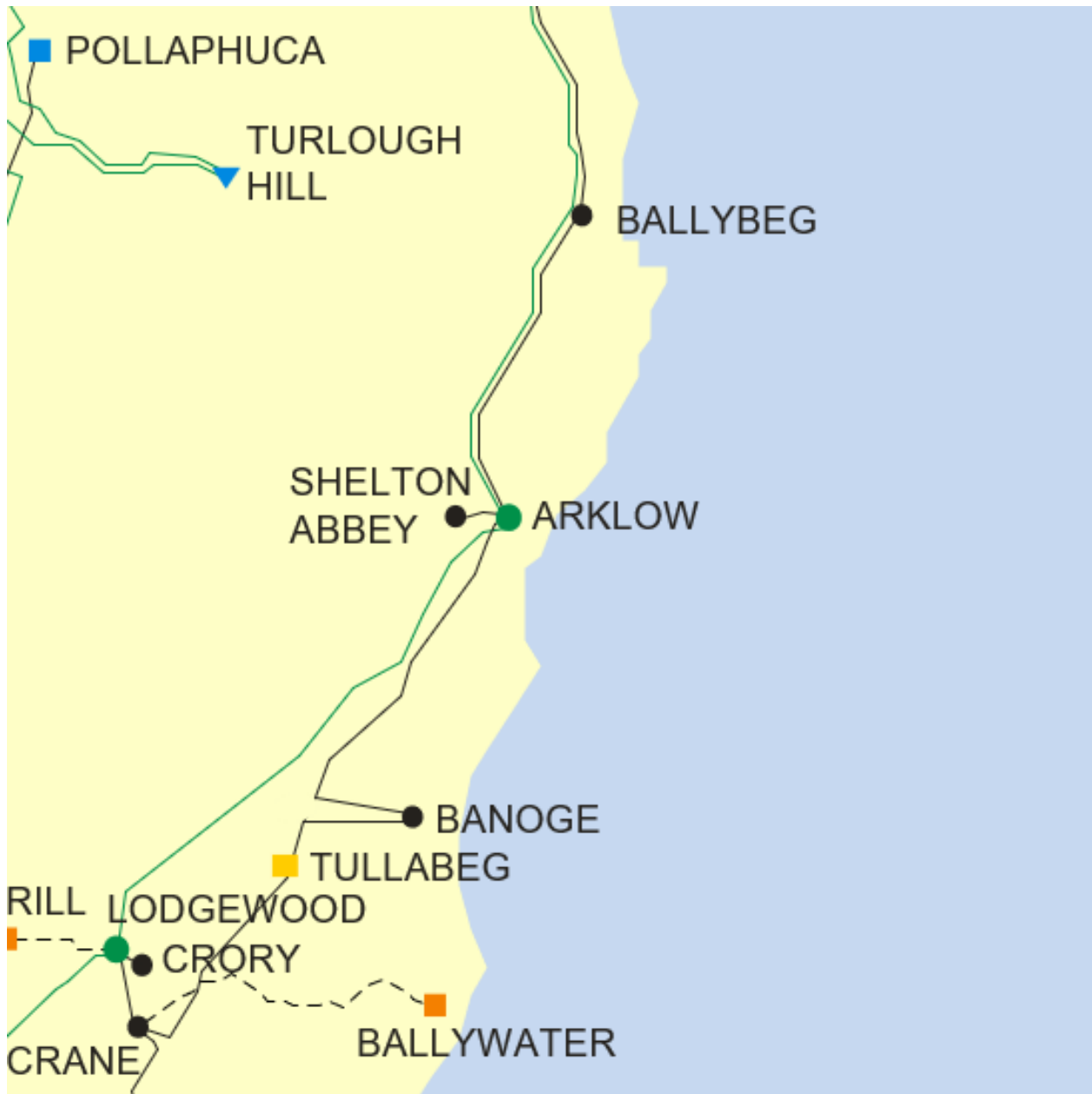
Figure 2-5 - Location of node Arklow 220 kV
