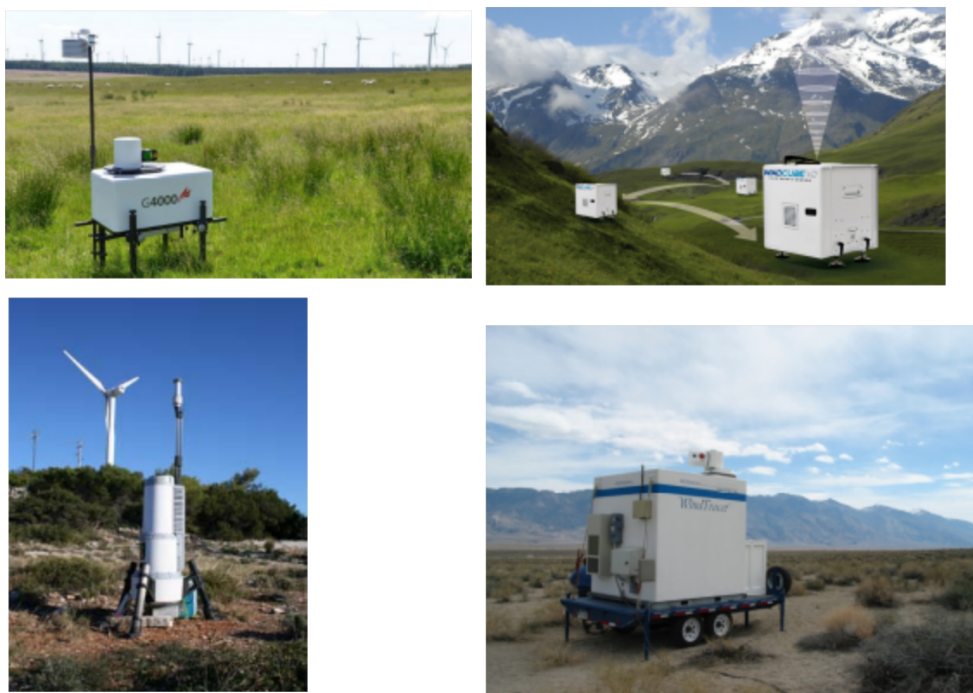
Figure 1.4: Examples of LiDARs for wind energy applications. Gallion (left top), Leosphere Windcube (right top), ZephIR (left bottom), Wind Tracer, Doppler LiDAR Lockheed Martin (right bottom).
