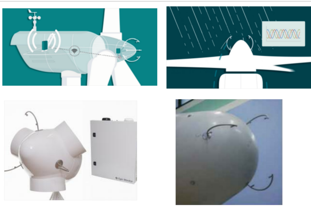
Figure 1.9: Ultra-sonic anemometer spinner technology iSpin from ROMO Wind as schematic and also an example of a nacelle top mounted from METEK (bottom right).
