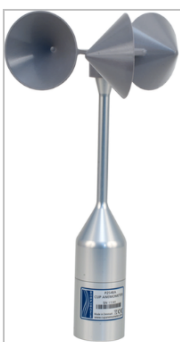
Figure 1.7: MEASNET certified cup anemometer from Campbell Scientific and a cup anemometer 40C from RNRG.
