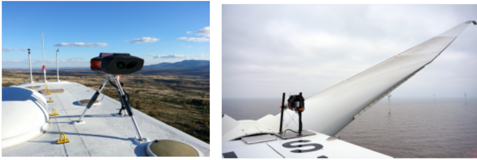
Figure 1.10: Example of nacelle mounted ZephIR LiDAR and METEK iSpin technology.
