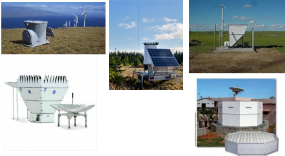
Figure 1.5: Examples of SODARs used in wind energy applications. Vaisala Triton (left top), AQ 510 , (middle top), ASC 4000i (top right), METEK PSC (bottom left), Scintec XFAS (bottom right).
