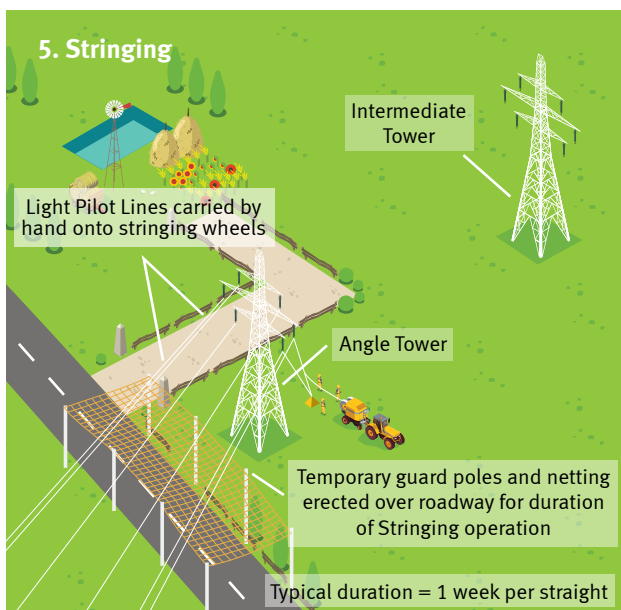
Figure 3.9: Tower construction summary
