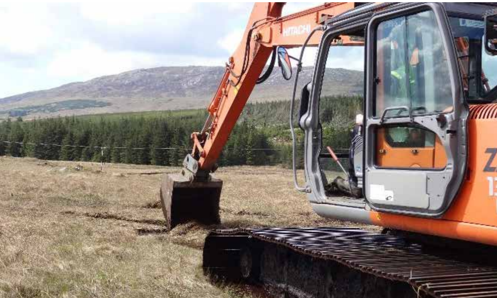
Figure 5.4: Wide-tracked low ground bearing machine
