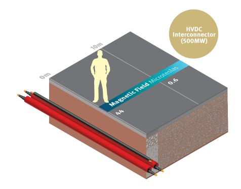
Figures shown are typical. Magnetic field levels will vary for each installation, and will vary depending on how much power is carried in the cable.
