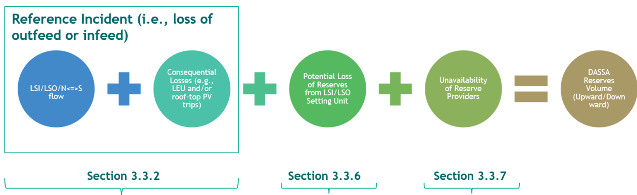
Figure 6: Overview of the factors contributing to the determination of required upward and downward reserves as discussed in this section 3.3.
