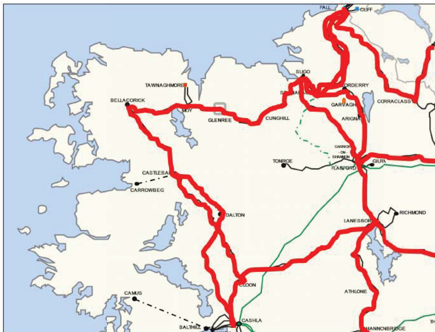
Figure ES1 - Map Illustrating the Overloaded Circuits in the Bellacorick Area
