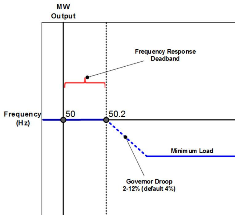
Figure PPM1.5.3.11: Limited Frequency Sensitive Mode – Over-frequency
