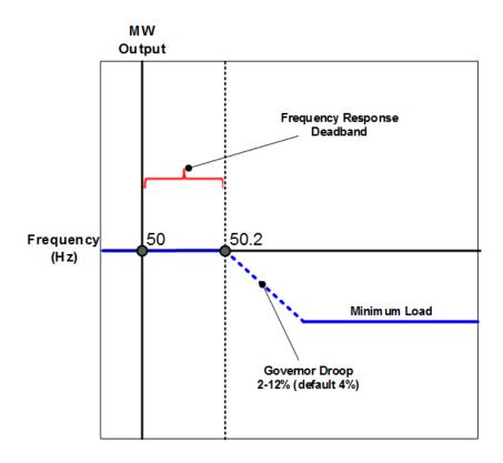
Figure OC.4.3.4.1.8: Limited Frequency Sensitive Mode – Over-frequency
