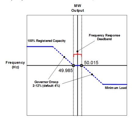
Figure OC.4.3.4.1.10: Frequency Sensitive Mode
