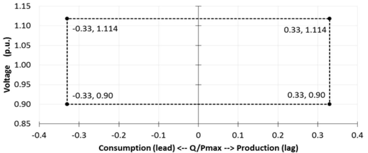
An **Interconnector** shall be capable of moving to any operating point within their U-Q/ $P_{max}$  profile, without undue delay, and shall be capable of moving from its minimum **Reactive Power** capability  $Q_{min}/P_{max}$  (Import/Lead) to its maximum **Reactive Power** capability  $Q_{max}/P_{max}$  (Export/Lag) within 120 seconds, depending on the **Active Power** output.
