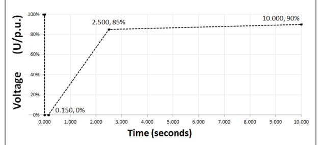
Figure CC.7.5.12: Voltage-against-time profile at the Connection Point for symmetric amd asymmetric fault conditions
