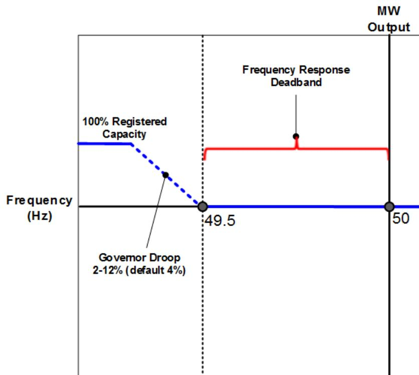
Figure OC.4.3.4.1.9: Limited Frequency Sensitive Mode – Under-frequency
