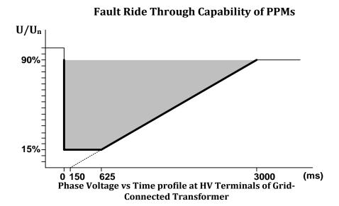
Figure PPM 1.1 - Fault Ride-Through Capability of Controllable PPMs
