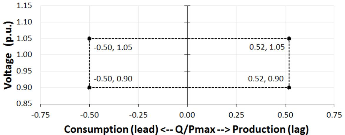
The **Generation Unit** shall be capable of moving to any operating point with its U-Q/P<sub>max</sub> profile in appropriate timescale to target values. The appropriate timescale shall be identified during the **TSO's Connection Offer** process.
