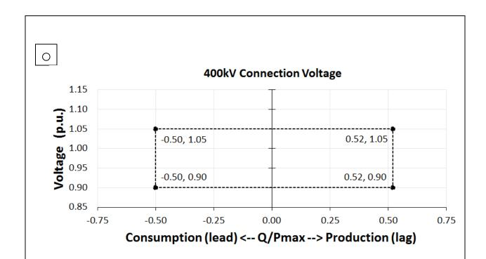
The **Generation Unit** shall be capable of moving to any operating point with its  $U-Q/P_{max}$  profile in appropriate timescale to target values. The appropriate timescale shall be identified during the **TSO's Connection Offer** process.
