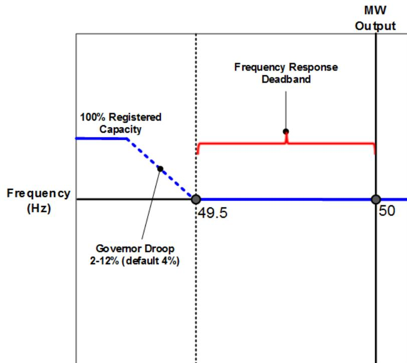
Figure PPM1.5.3.12: Limited Frequency Sensitive Mode – Under-frequency
