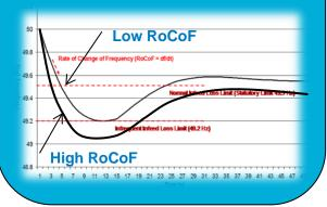
In the future with increasing the level of non-synchronous generation (i.e. solar PV, windfarms) the system inertia will reduce
