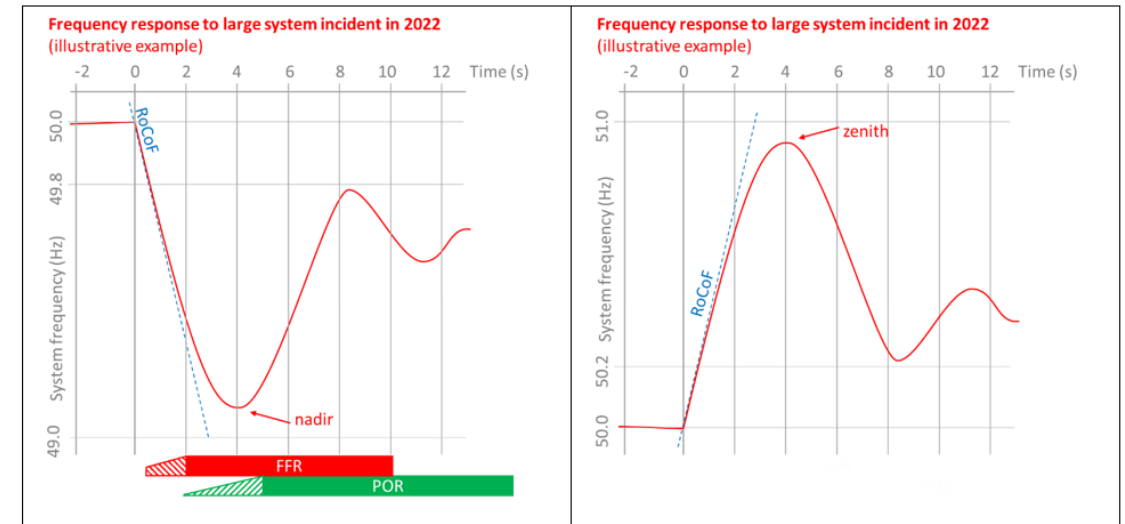
Figure 6 Illustrative example of a frequency trace following loss of largest single infeed (left) and largest single outfeed (right) in 2022
