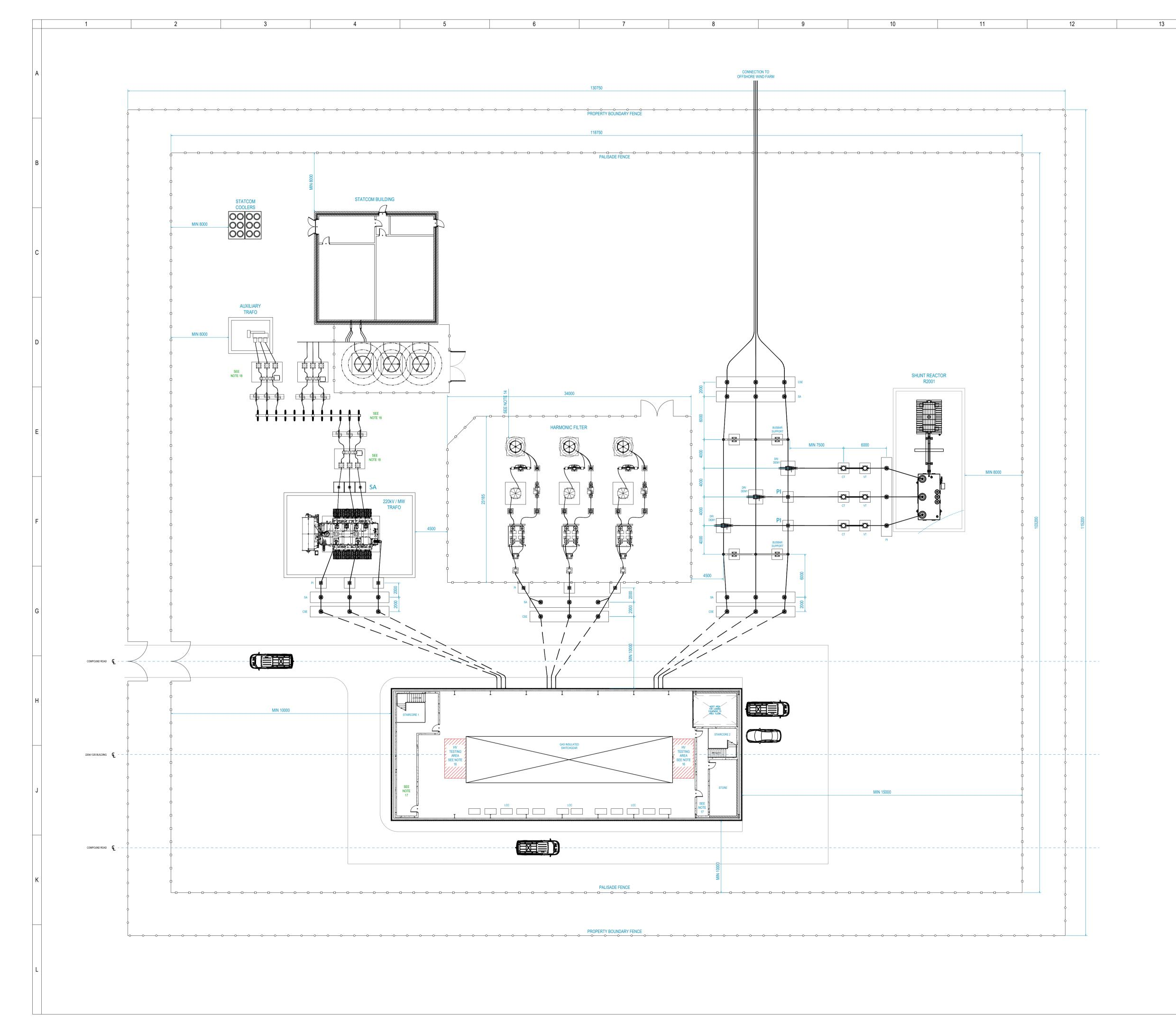
THIS CONCEPTUAL DESIGN IS BASED ON A FULL 8 BAY GIS WITH SECTIONALISER AND WING COUPLERS (A STANDARD GIS BUILDING). IT IS ACKNOWLEDGED AND ACCEPTED THAT AN ONSHORE COMPENSATION COMPOUNDS CAN BE SINGLE BUSBAR WITHOUT SECTIONALISERS. IT IS EXPECTED THE CUSTOMER WILL OPTIMISE THE LAYOUT FOR THEIR DEVELOPMENT.
