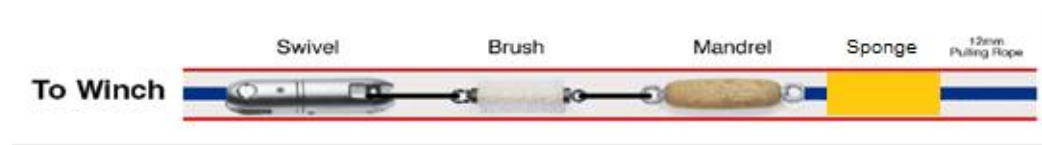
Figure 4 Set up for Swivel, Brush, Mandrel and Sponge for Duct Proving and Cleaning
