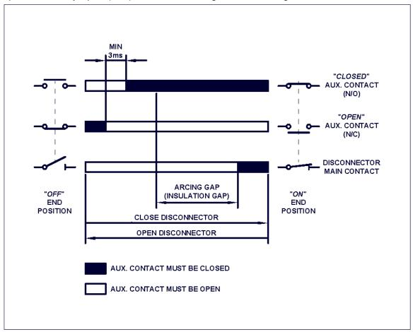
During the closing operation the N/O contact must close before the main contact reaches the insulation breakdown gap. During the opening operation the N/O contact ("Closed" signal) must not open before the main contact has passed the contact gap at which reignition can occur.
