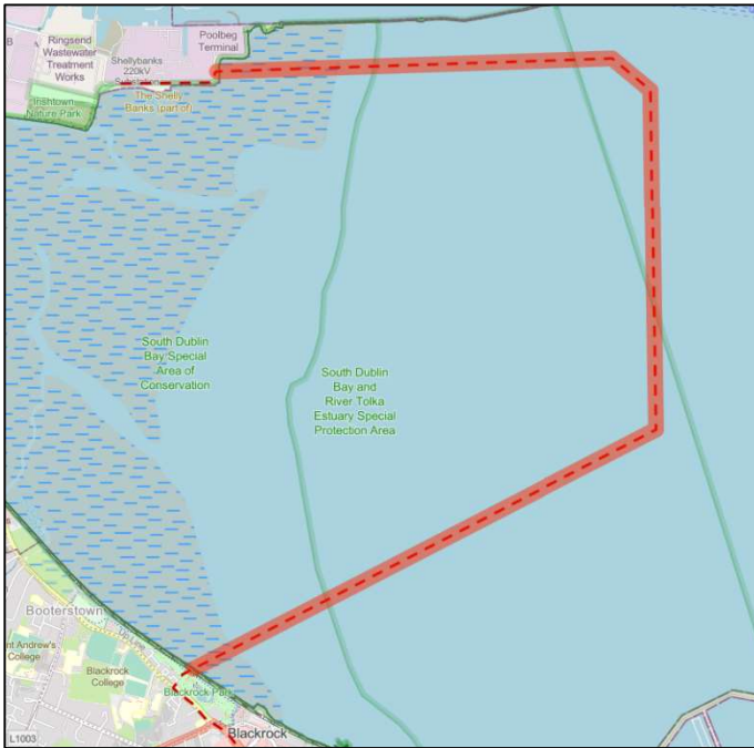
Figure 5-9: Best Performing Option: Submarine cable from Blackrock Park to Shelley Banks car park
