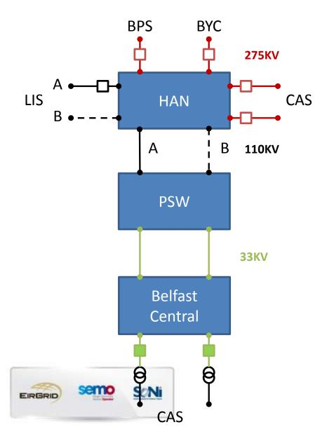
07:31 Lisburn A trips on overcurrent protection caused by the morning load lift
