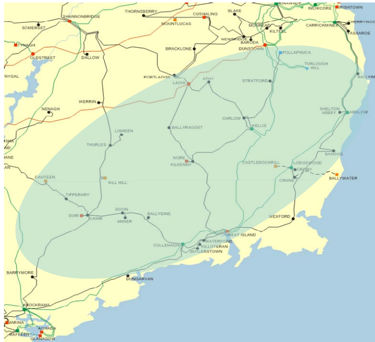
Figure 2.2: Illustration of the Extent of the Network Capacity Problems and the Voltage Support Requirements in a Future Planned Network
