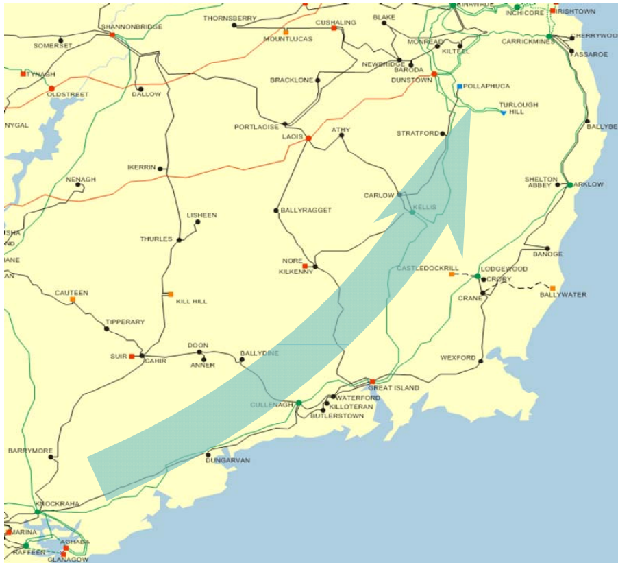
Figure 2.1: Map Showing the Electricity Power Flow from the South of Ireland towards the Dublin Area in a Future Planned Network
