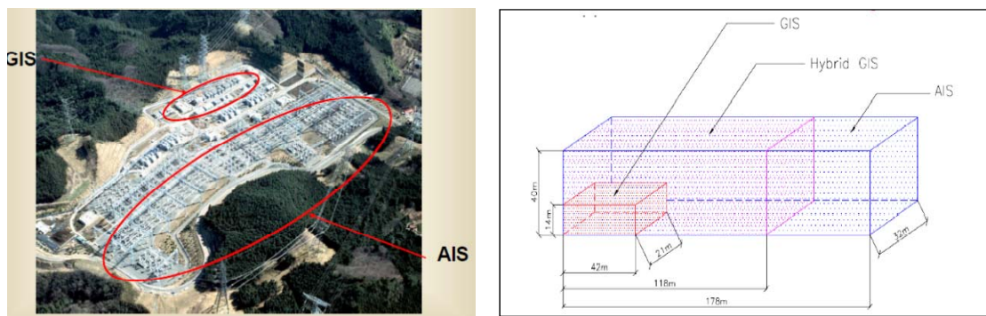
Figure 16: GIS vs. AIS Equivalent Substation Layouts
