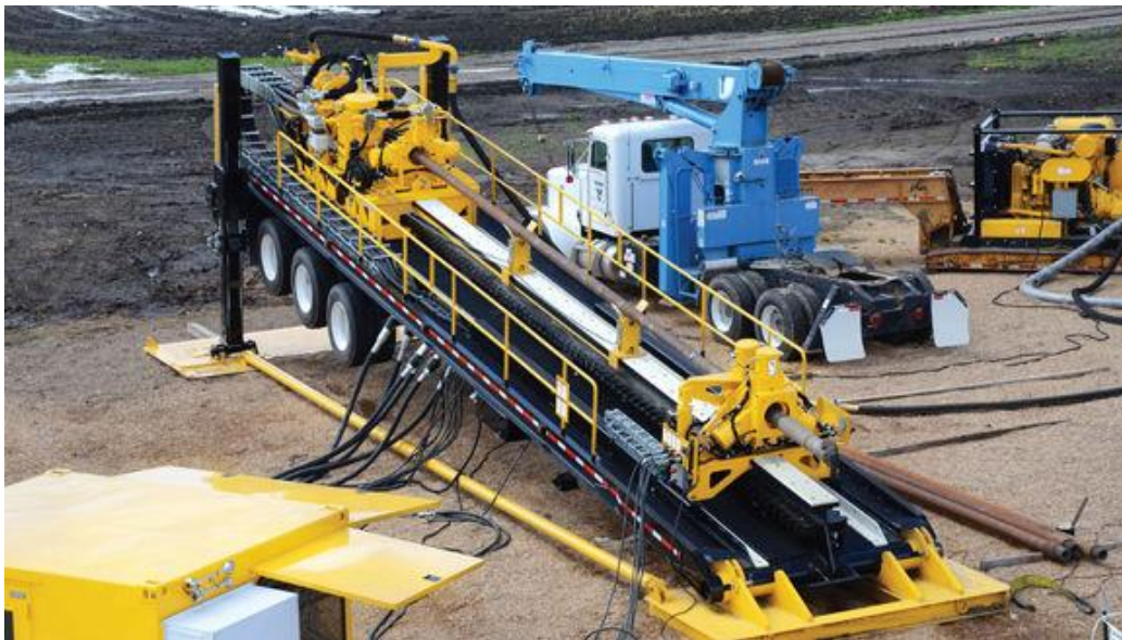
Figure 4.5: Typical HDD Drilling Rig
