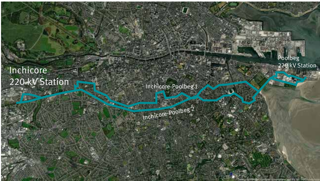
Figure 12: Inchicore-Poolbeg 1 & 2 220 kV Cables (Note: the alignments shown are the existing cable routes; routes for the replacement cables have not yet been identified)
