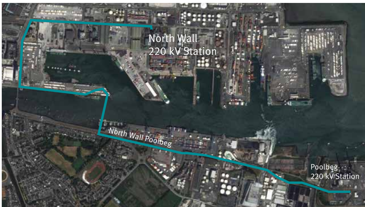
Figure 9: North Wall-Poolbeg 220 kV Cable (Note: the alignment shown is the existing cable route; a route for the replacement cable has not yet been identified)
