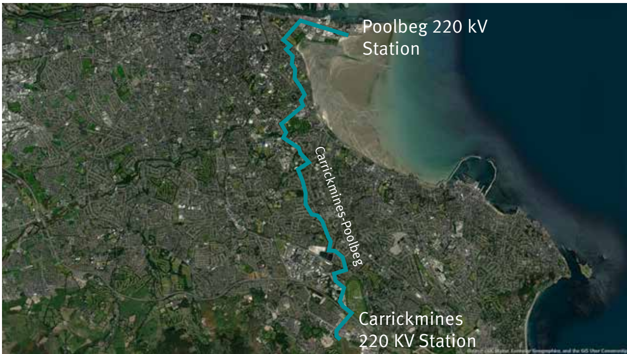
Figure 11: Carrickmines-Poolbeg 220 kV Cable (Note: the alignment shown is the existing cable route; a route for the replacement cable has not yet been identified)
