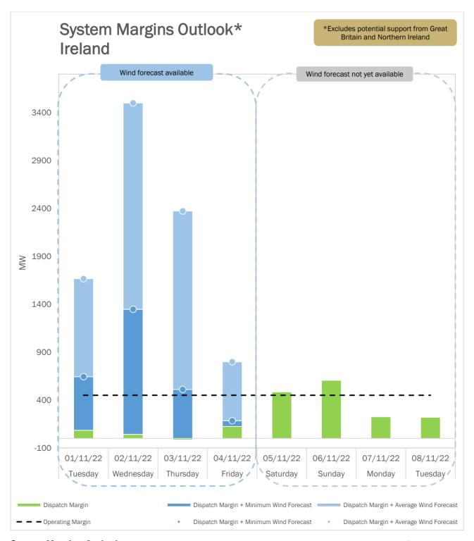
When a negative dispatch margin coincides with a low wind forecast, the net wind generation value may appear below the zero axis (low forecast: •, average forecast: •). It should be noted that the Daily Dispatch Margin and wind generation forecast are highly variable. The outlook is based on **estimates** and is therefore subject to rapid changes.
