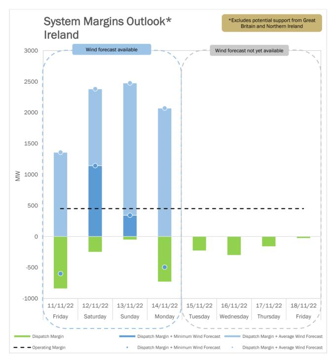
When a negative dispatch margin coincides with a low wind forecast, the net wind generation value may appear below the zero axis (low forecast: •, average forecast: •). It should be noted that the Daily Dispatch Margin and wind generation forecast are highly variable. The outlook is based on **estimates** and is therefore subject to rapid changes.
