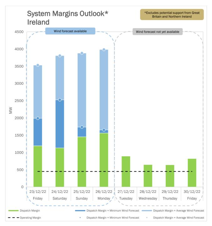
When a negative dispatch margin coincides with a low wind forecast, the net wind generation value may appear below the zero axis (low forecast: •, average forecast: •). It should be noted that the Daily Dispatch Margin and wind generation forecast are highly variable. The outlook is based on **estimates** and is therefore subject to rapid changes.
