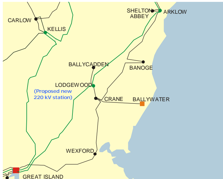
Figure D-3 Proposed Lodgewood 220 kV Station
