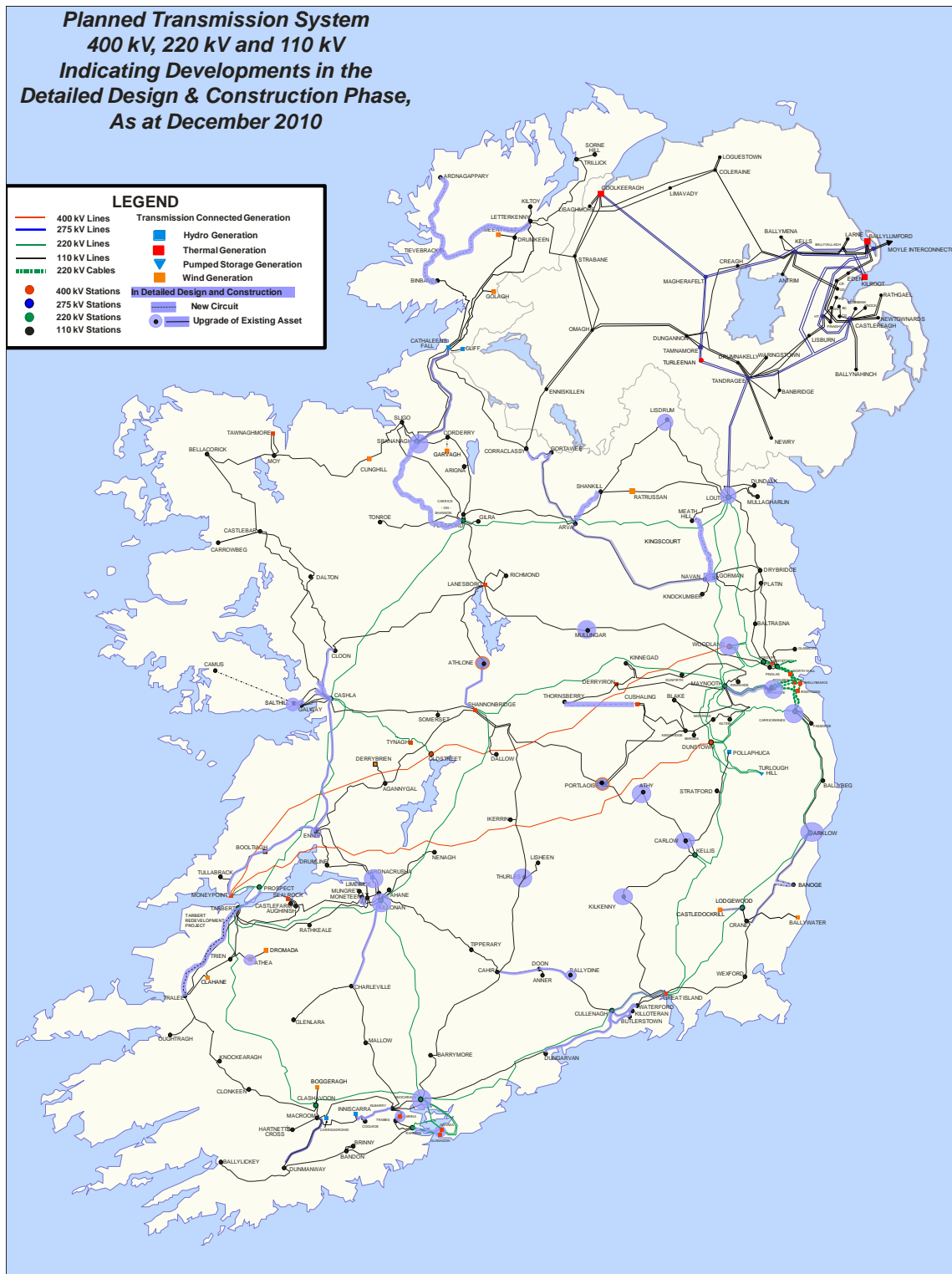
Figure A2 Map Indicating Planned Network Developments in the Detailed Design & Construction Phase
