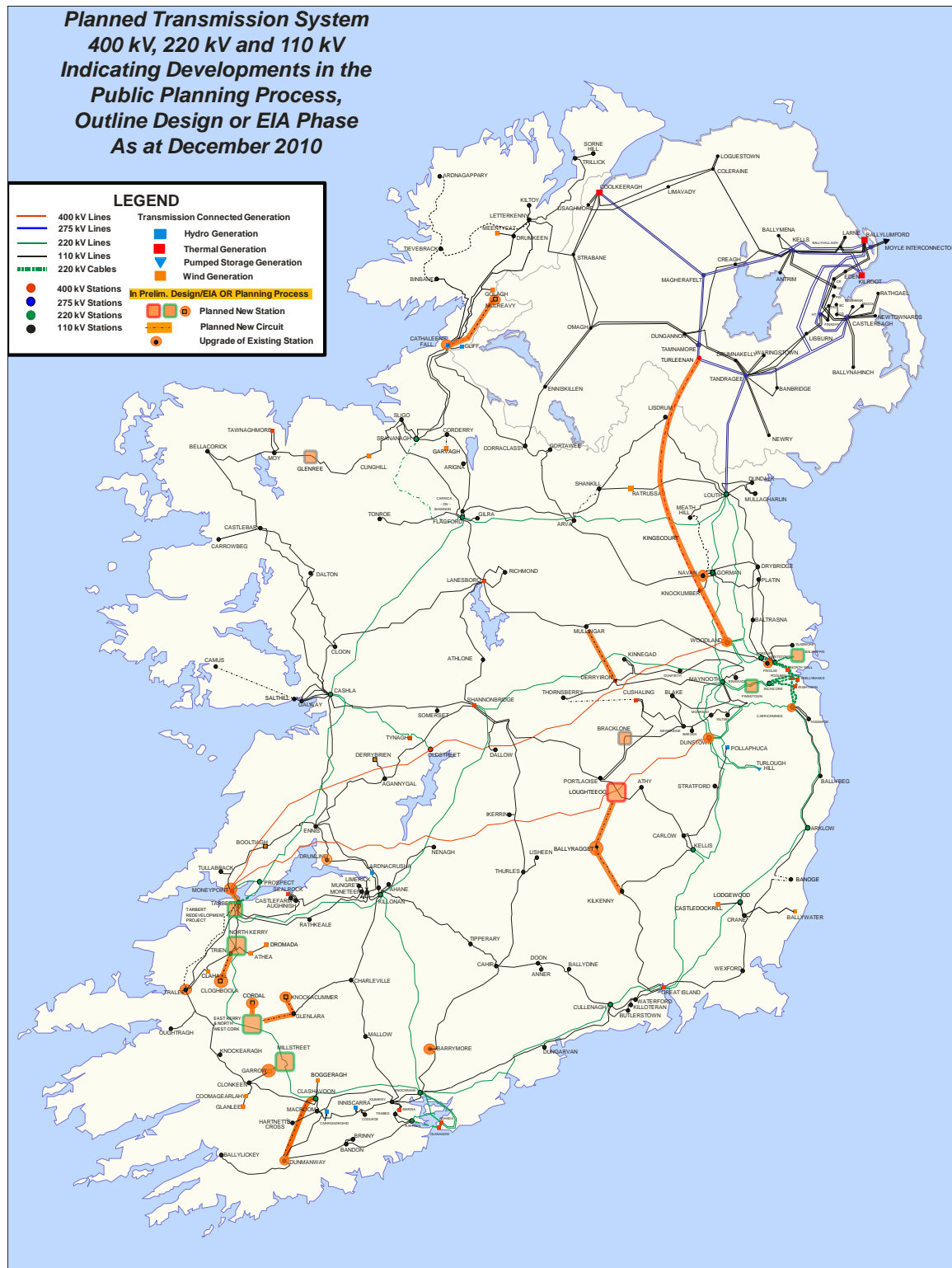
Figure A3 Map Indicating Planned Network Developments in the Outline Design Phase and Public Planning Process Note: All new developments on this map are subject to existing/on-going EIA
