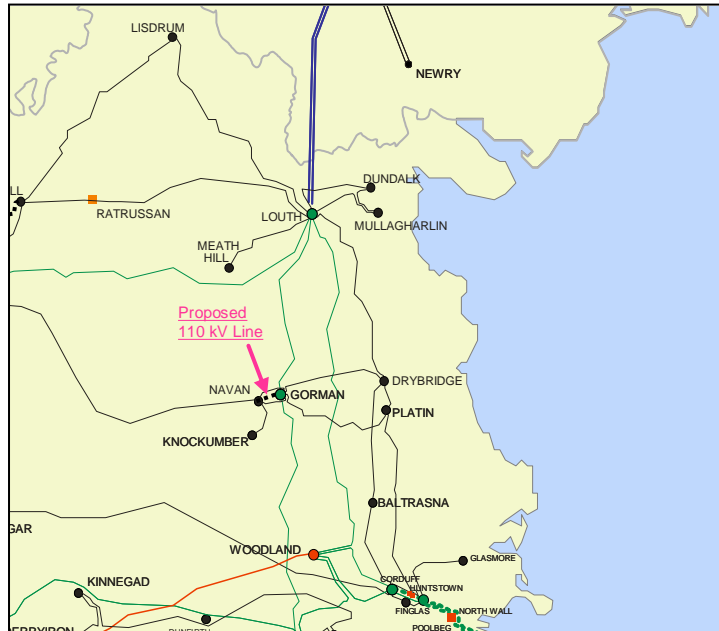
Figure B-9 Proposed Gorman-Navan No.3 110kV line
