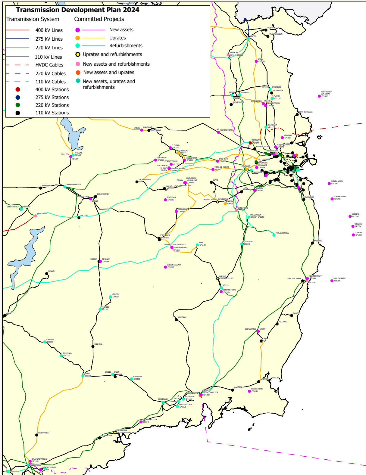
Figure 5-3 (a): Planned network developments in Steps 4 to 6 in the Southeast, Mideast and Dublin
