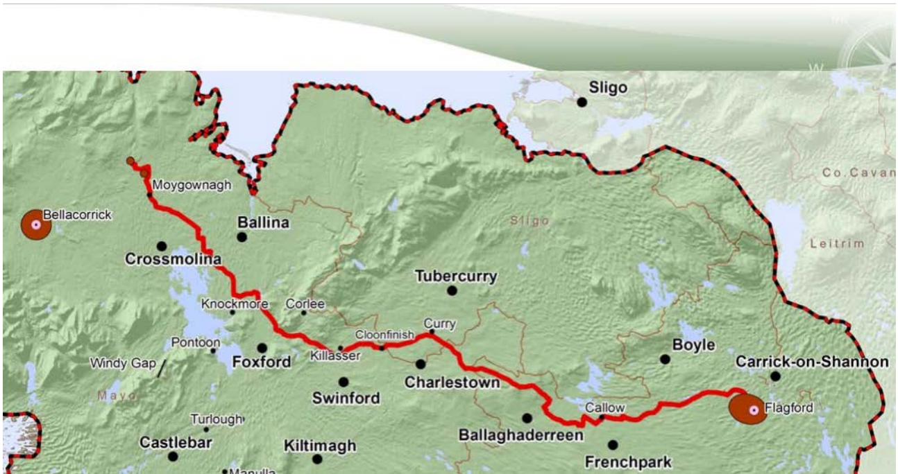
Figure 8.1 Underground Route Option A
