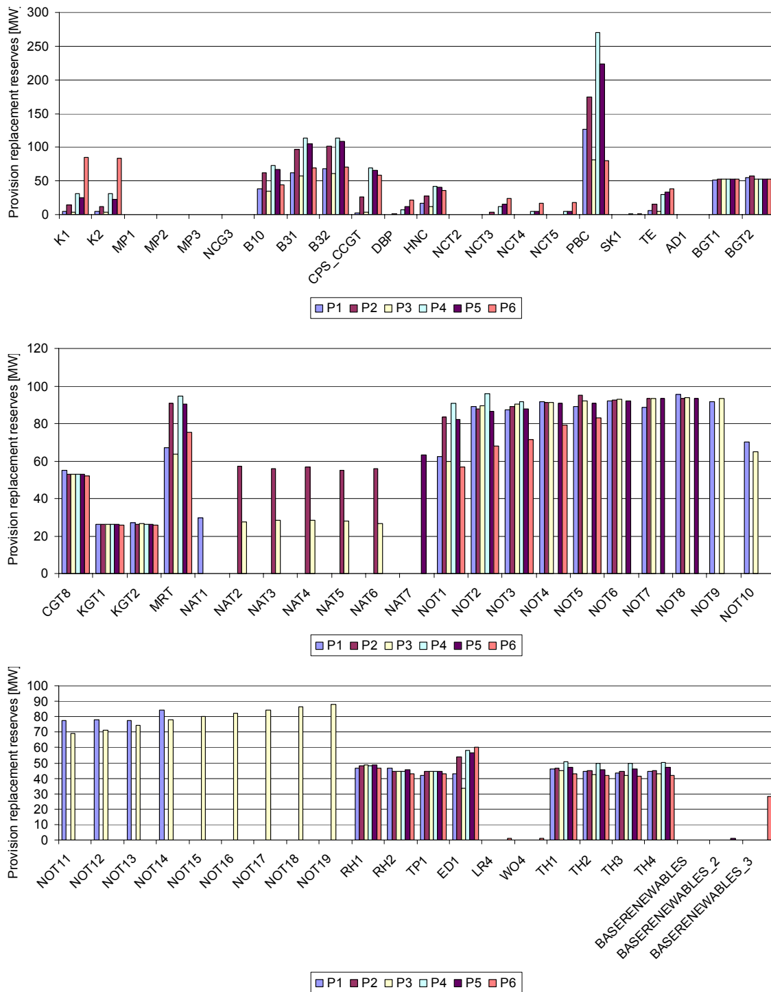
Figure 19. Hourly supply of replacement reserves distributed on units and averaged over the year.
